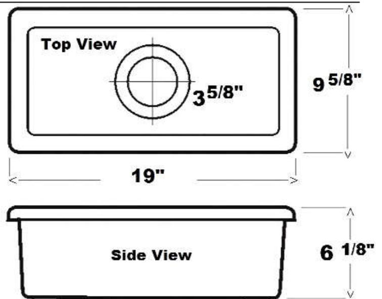
Dimensions of fixture are nominal and may vary within the range of tolerances established by ANSI Standard A112.19.9. Dimensions and specifications subject to change without notice.
