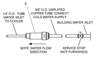
Figure 17 – Water Supply Connections
