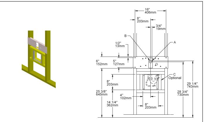
Figure 1 - Rough-in for EDFPB114C W/MP86 Mounting Plate
