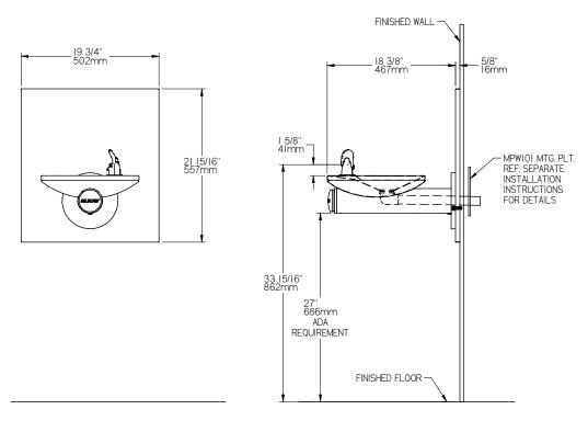
Figure 6 -Rough-in Assembly EDFPB(V)114C W/MPW101 MOUNTING PLATE
