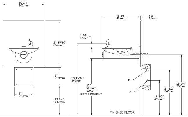
Figure 4 - Rough-in Assembly for EDFPBWM114C
