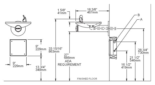
Figure 2 - Rough-in Assembly For EDFPB114C
