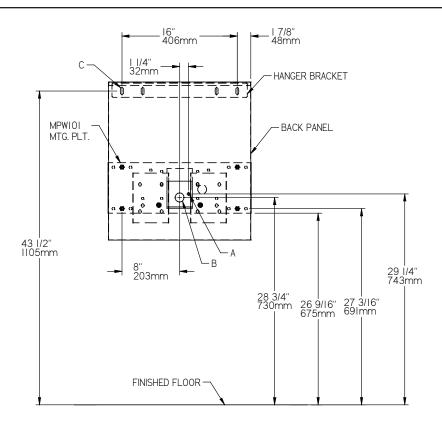
Figure 5 -Rough-in EDFPB(V)114C W/MPW101 MOUNTING PLATE
