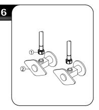
Make connections to water lines. Thread the nut (1) on the supply line onto the outlet of the water supply valve (2) and tighten with a wrench. Do not overtighten.
