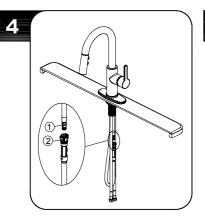
Align male fitting (1) and tabs (2) on quick connector. Push quick connector housing firmly upward and snap onto receiving male fitting. Pull down moderately to ensure connection has been made.
