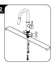
Optional Deck Plate Installation: Before installation, align the hole in the gasket (1) and deck plate (2) with the mounting hole in the sink. Place the faucet assembly through the deck plate (2) and mounting hole in the sink until the faucet assembly sets on top of deck plate (2). NOTE: If the sink is uneven, use silicone
