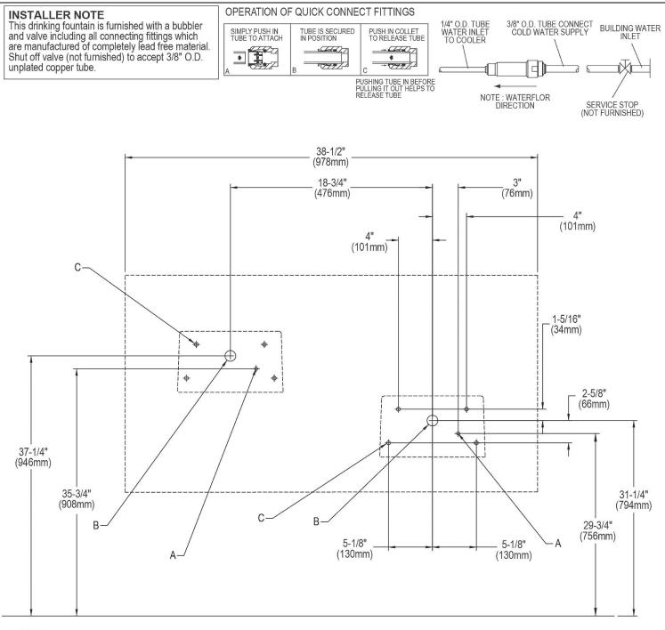
LEGEND A = 7/8" (22mm) Ø Hole for water supply tube B = 1-3/4" (44mm) Ø Hole for waste line C = 1/2" (13mm) Ø Clearance hole for mounting
