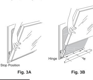
When the door is removed and hinge arms are at stop position, do not bump or try to move the hinge arms. The hinges could snap back causing an injury to the hands or damage to the porcelain on the front of the range. Cover the hinges with toweling or empty towel rolls while working in the oven area.
