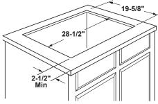
Dimension and installation information are shown in inches. \*Allow 5-3/4" depth at rear for electrical and gas connections
