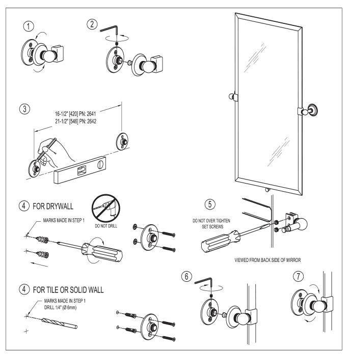
**Tools needed:** Pencil, Tape measure, Phillips Screwdriver, Drill and Level.
