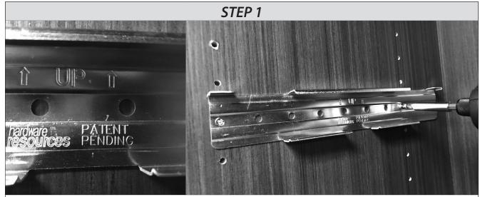
Determine mounting location and install the mounting bracket with the arrows pointing up with the 5 mm Euro screws provided.
