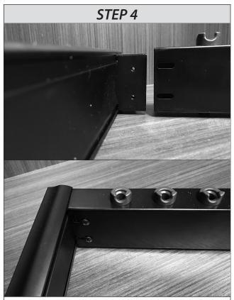
Install Cross Member to Slide Cover by sliding the angle brace inside the Cross Member making sure the slotted pant hanger holders are pointing upward. Loosely fasten with 2 – Pan Head Machine screws provided.
