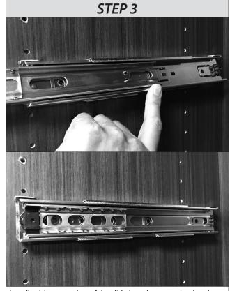
Install cabinet member of the slide into the mounting bracket. Angle the top in first and then snap into place.
