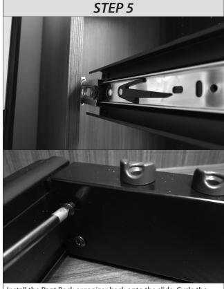
Install the Pant Rack organizer back onto the slide. Cycle the unit a couple of times to be sure it is not binding, allowing the Cross Member to center between the Slide Covers. Securely tighten the machine screws.
