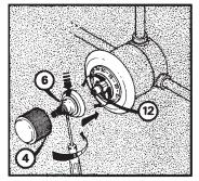
Let the water flow and bring this to a mean temperature by actuating the bushing (12). Note this temperature. Place the pointer assembly (6) on the bushing and position the "red" index opposite the graduation corresponding to the temperature noted.
