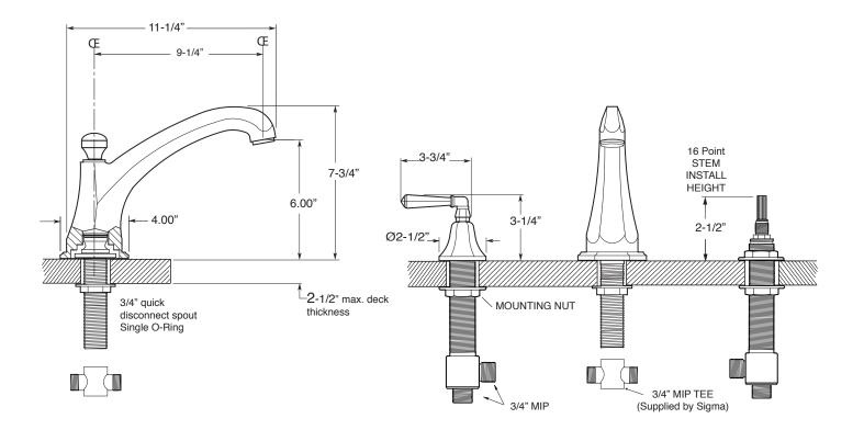
NOTE: Spout and valves install through 1-1/4" diameter holes. Plumber to provide 3/4" supply lines to valves
