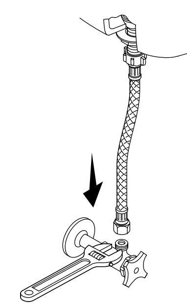
17A. Turn on the water supply and adjust the water level. Flush the toilet and recheck the water level.
