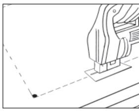
3. Using a saber saw, cut inside of the cutout line. Trial fit to check for proper fit.
