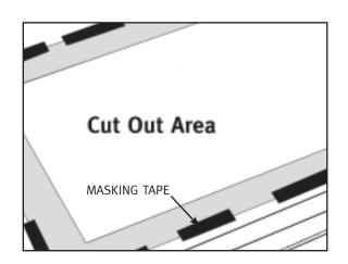
**1.** Cut out the inside of the template. Locate the template front to rear and right to left on the countertop. Make sure that the bowl location will not interfere with the cabinet below or the plumbing. Attach the template to the countertop with masking tape and draw a pencil line around the inside of the template.
