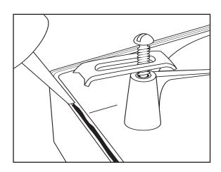
**4.** For final fit, apply a bead of caulk (not included) to the underside of the sink flange and position onto the countertop opening. First, tighten screws in front, and then tighten rear screws.
