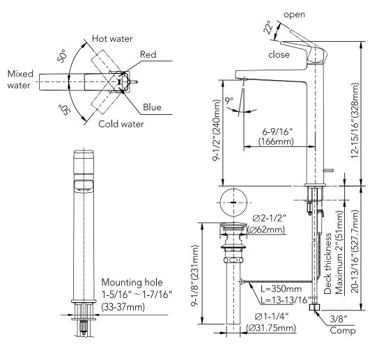
NOTE: The above dimensional unit is inch. The dimension in ( ) is reference mm.
